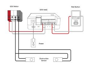
First, remove the wall button wires from the red and white terminals on the back of the motor unit and reconnect them to the red and white terminals labled WALL BTN on the Konnected device.
