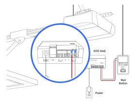
To mount on near the wall button, leave all existing wires in-place and connect one end of the red and white wires to the corresponding screws marked RED and WHITE (or R and W) on the back of the wall button, and the other end to the red and white terminals marked
